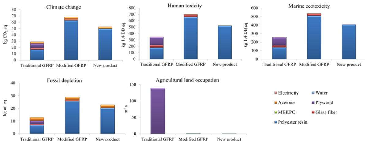
Fig. 3 Environmental impacts of traditional GFRP, modified GFRP and new product related to raw materials used for a 1x1 m<sup>2</sup> table top with 1 cm thickness
