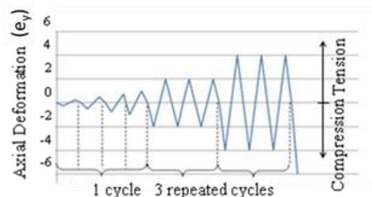
Fig.3 Cyclic loading scheme
