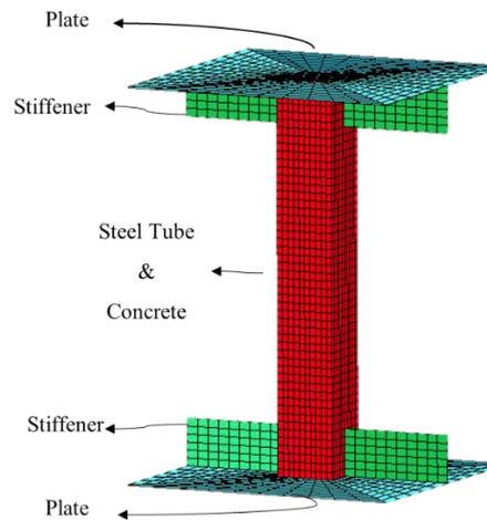
Fig.4 Finite element model
