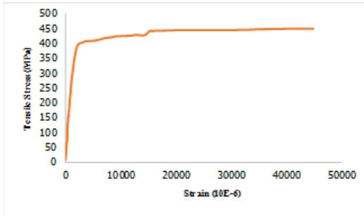
(b) Steel tube with 3 mm thick
