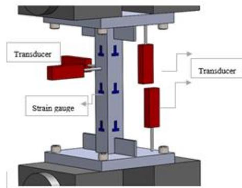
Fig.2 Installation of specimen to testing machine
