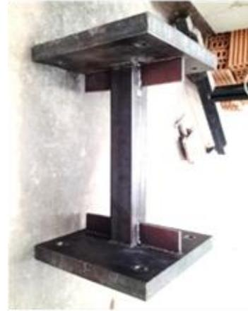
Fig.1 Test specimen with bearing plate machine.
