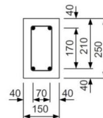
Fig.2 Dimension of the tested beam sample
