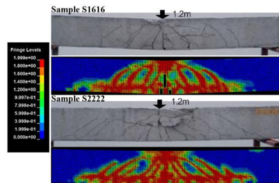
Fig.6 Crack pattern comparisons (Numerical simulation and Experimental results)
