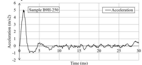
Fig.8 Midspan acceleration of sample B9H-250
