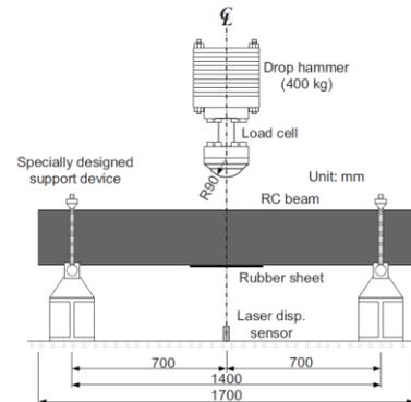
Fig.1 Tested setup used in Fujikake's work [3]
