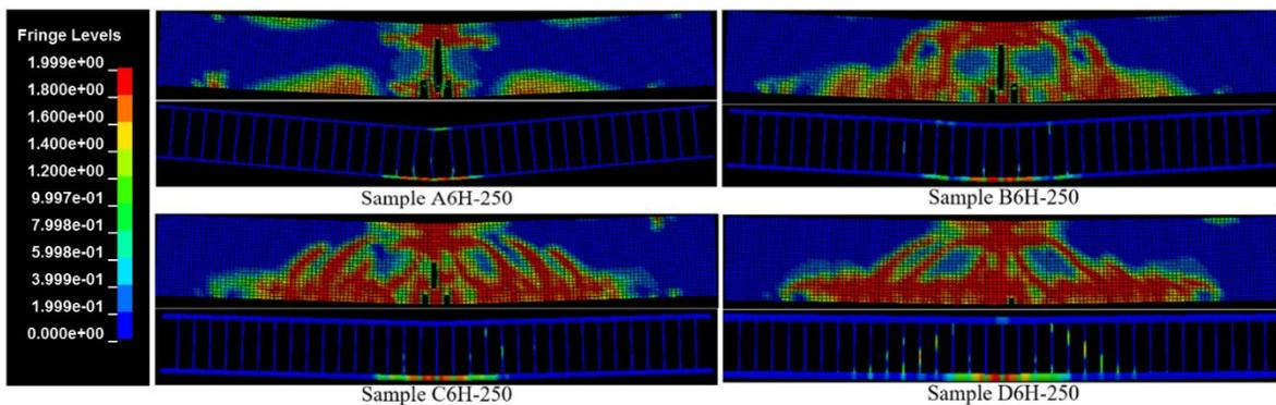
Fig.9 Examples of crack pattern and plastic strain in reinforcement of RC beams
