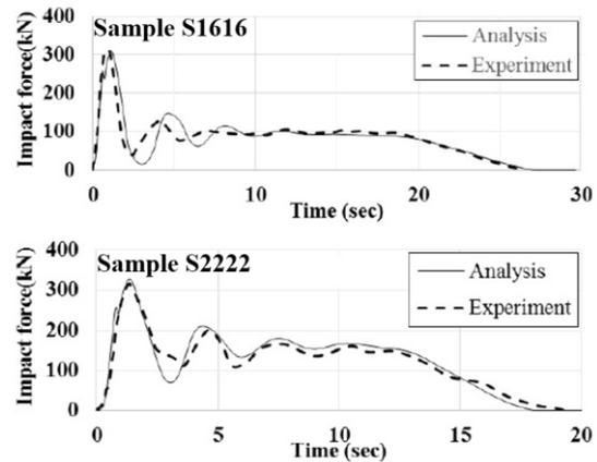
Fig.4 Impact force comparisons (Numerical simulation and Experimental results)
