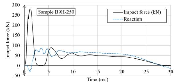
Fig.7 Impact force and reaction force at supports of sample B9H-250
