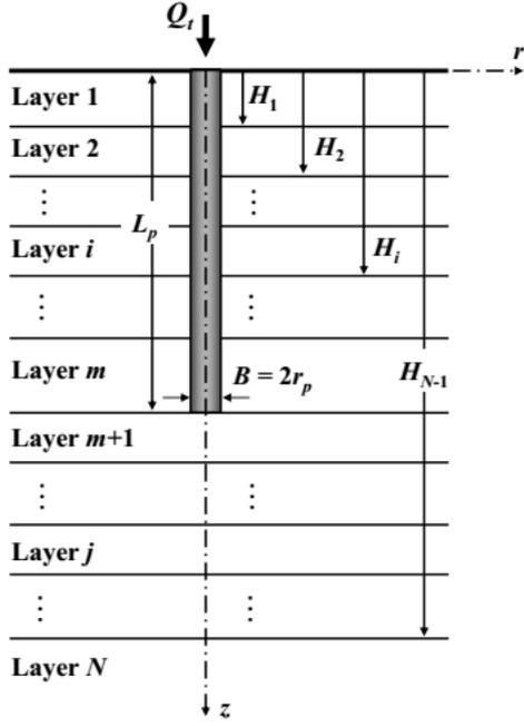
Fig. 1 Axially loaded pile and multi-layer soil, modified from [5]
