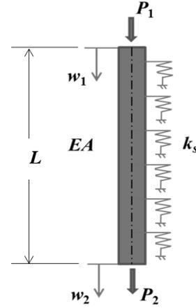
Fig. 2 Axially loaded pile element and element degrees of freedom, modified from [4]
