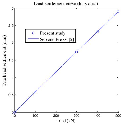
Fig. 6 Load-settlement curve at pile head (Italy case)
