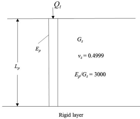
Fig. 3 Pile rest on rigid layer, modified from [6]
